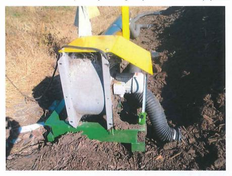
225/6 MAF blower housing in galvanised steel and manifold pipework in heavy poly pipe
