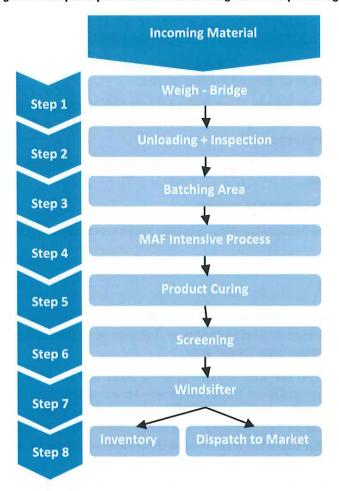
Figure 4-1: Proposed process flow schematic diagram for the processing of FOGO material at DWM
