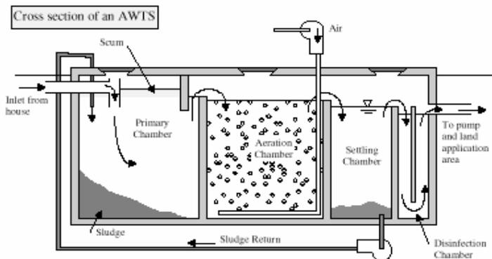
flows into a second chamber. Here the wastewater is mixed with air to assist bacteria to further treat it. A third chamber allows additional clarification through the settling of solids, which are returned for further treatment to either the septic chamber (as shown) or to the aeration chamber. The clarified effluent is disinfected in another chamber (usually by chlorination) before irrigation can take place.
